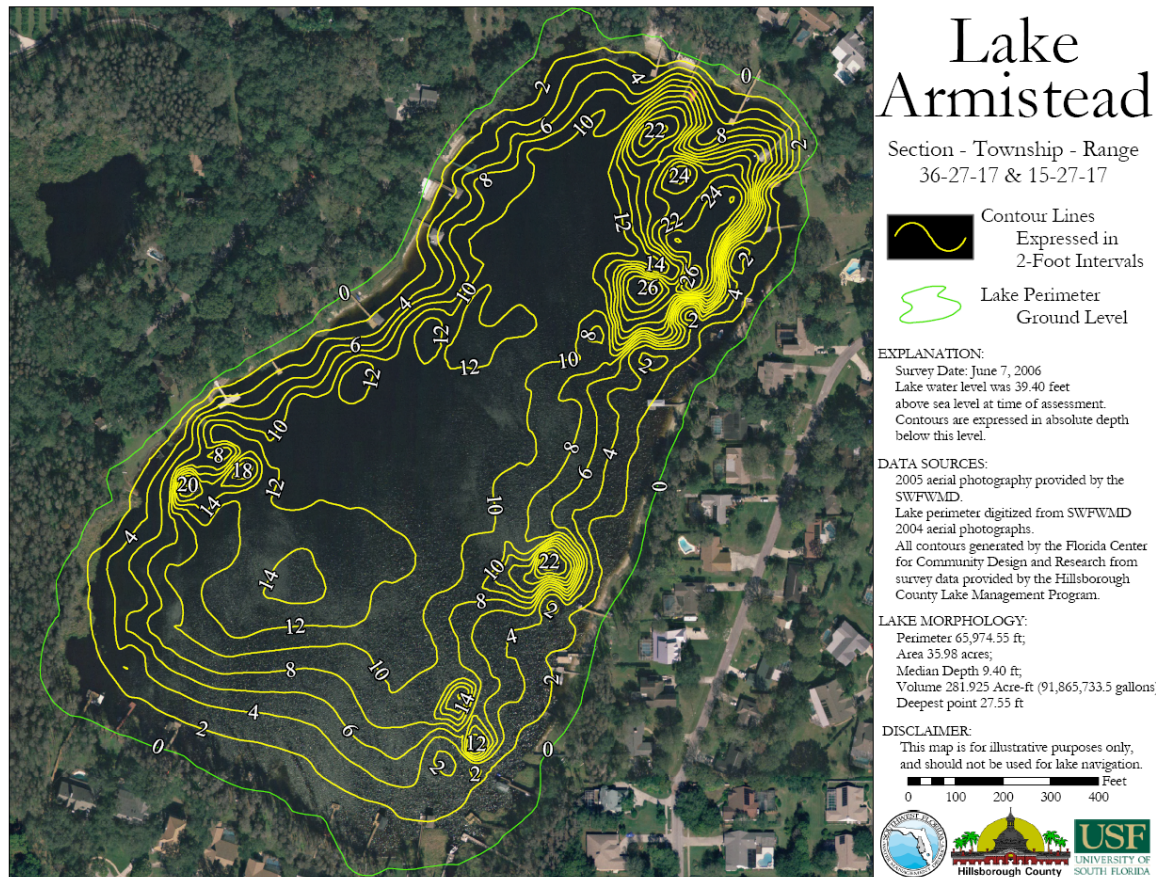
Figure 2. Contour map for Lake Armistead. The lake was mapped during the 2006 lake assessment project. A differential global positioning system and fathometer combination instrument was used to obtain simultaneous horizontal and vertical measurements.
