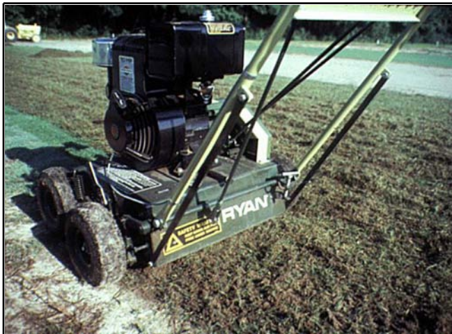
Figure 8. Removing Thatch with a Vertical Lawnmower (Verticutting)
